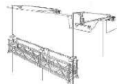
Max load: 150kg/m 2 In system construction: additional lock on fixtures In pipe & coupling construction: additional cross-coupling No swivel couplers for load-bearing elements
